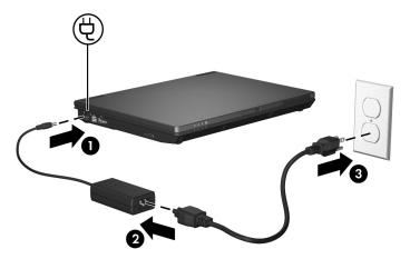
When the computer receives AC power, the battery begins to charge and the battery light (on the front of the computer) turns on. When the battery is fully charged, the battery light turns off.
